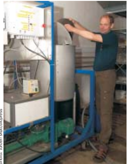
Henrik B. Møller pours liquid manure into the pretank of one of the four test reactors in the liquid manure labora-
