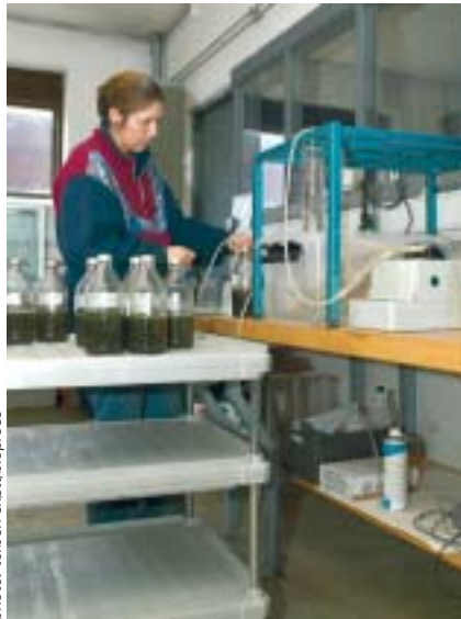
Laboratory technician Gitte Hastrup Andersen carries out a test where energy crops are degassed.
