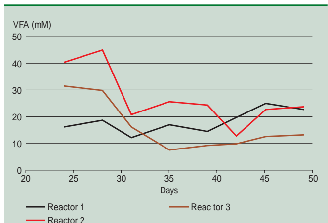
Figure 3. The VFA concentration of three test reactors. Cattle manure was used, and the tests were carried out at a process temperature of 55°C.
