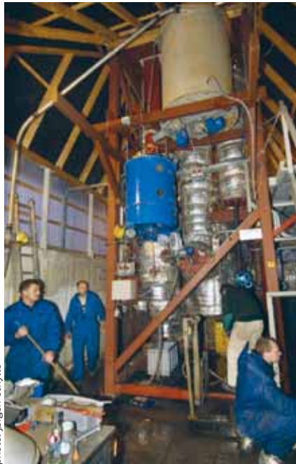
The 500 kW gasification plant at the Technical University of Denmark.
