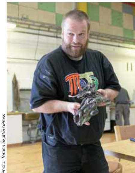
Thomas Koch holding a handful of slag stemming from a waste water sludge gasification process. The slag may be utilised in the production of concrete, table tops, filling material for road surfaces, etc.
