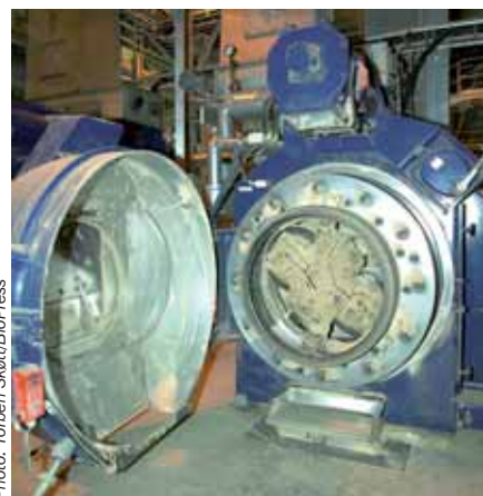
Rotating pellets press at Køge Biopillefabrik. A large part of the trials carried out at the Institute of Mechanics, Energy and Construction involved a similar, although smaller, press.
