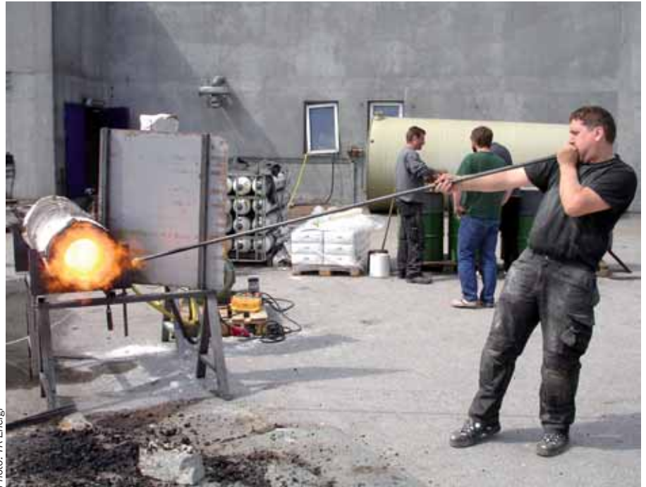
Testing a small trial plant for waste gasification at TK-Energi in Køge. The picture shows a test run on the slag produced by the plant.
